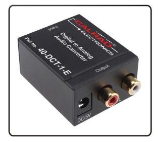
The 40-DCT-1-E converts a digital audio signal source from a digital coax RCA jack or optical toslink jack and converts to an analog stereo audio signal L+R RCA output jacks. Compact size and easy to install.
